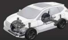
MacPherson Strut & Multi Link Suspension
